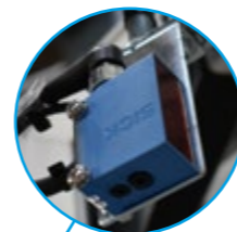
Anti-collision safety photocells for descent movement
