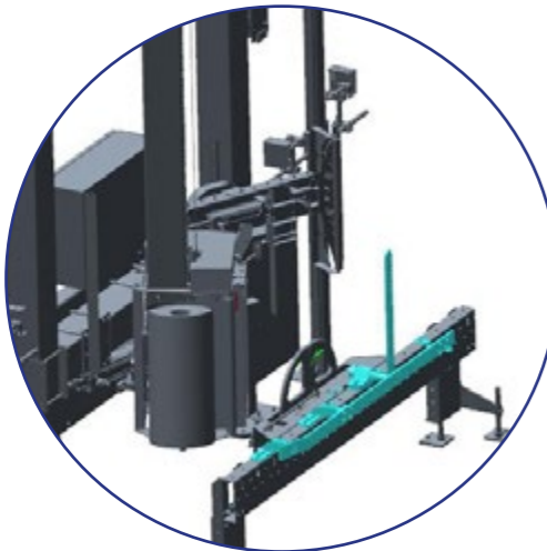
Fixed welding backing plate
