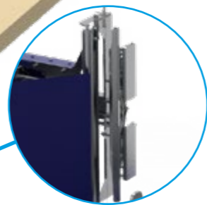
Film cutting and sealing unit moun- ted on the machine base
