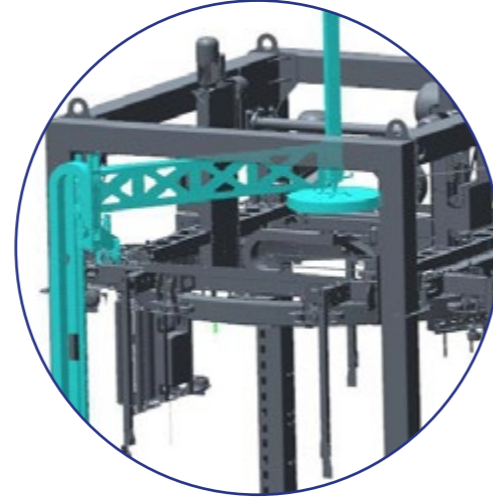
Gravity stabilizer press + cylinder for feeder passage
