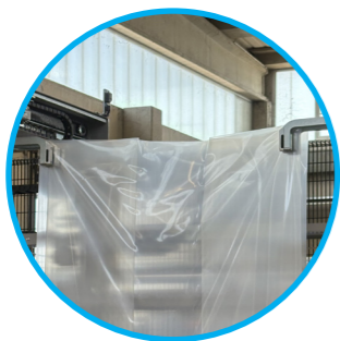
System for gripping and opening the elastic hood
